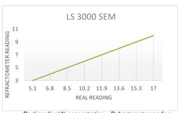
Real reading/ % concentration = Refractometer reading x refractive factor.
