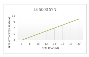
Real Reading / % concentration = Refractomer reading x refractive factor.
